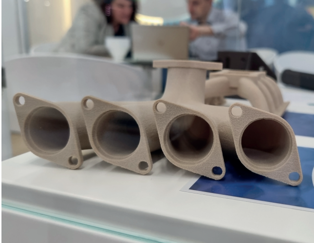
Fig. 5. In future, the PAEK introduced by Solvay is said to permit components made of the high-performance thermoplastic to be printed at lower temperatures. © Hanser/F. Streifinger
