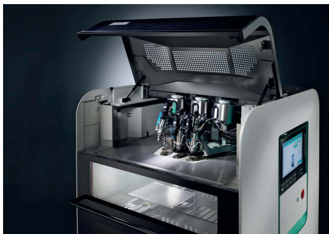
Fig. 2. The three discharge units of the Freeformer 750-3X have a more compact design than the 300-3X version, and can therefore be arranged more closely together.
