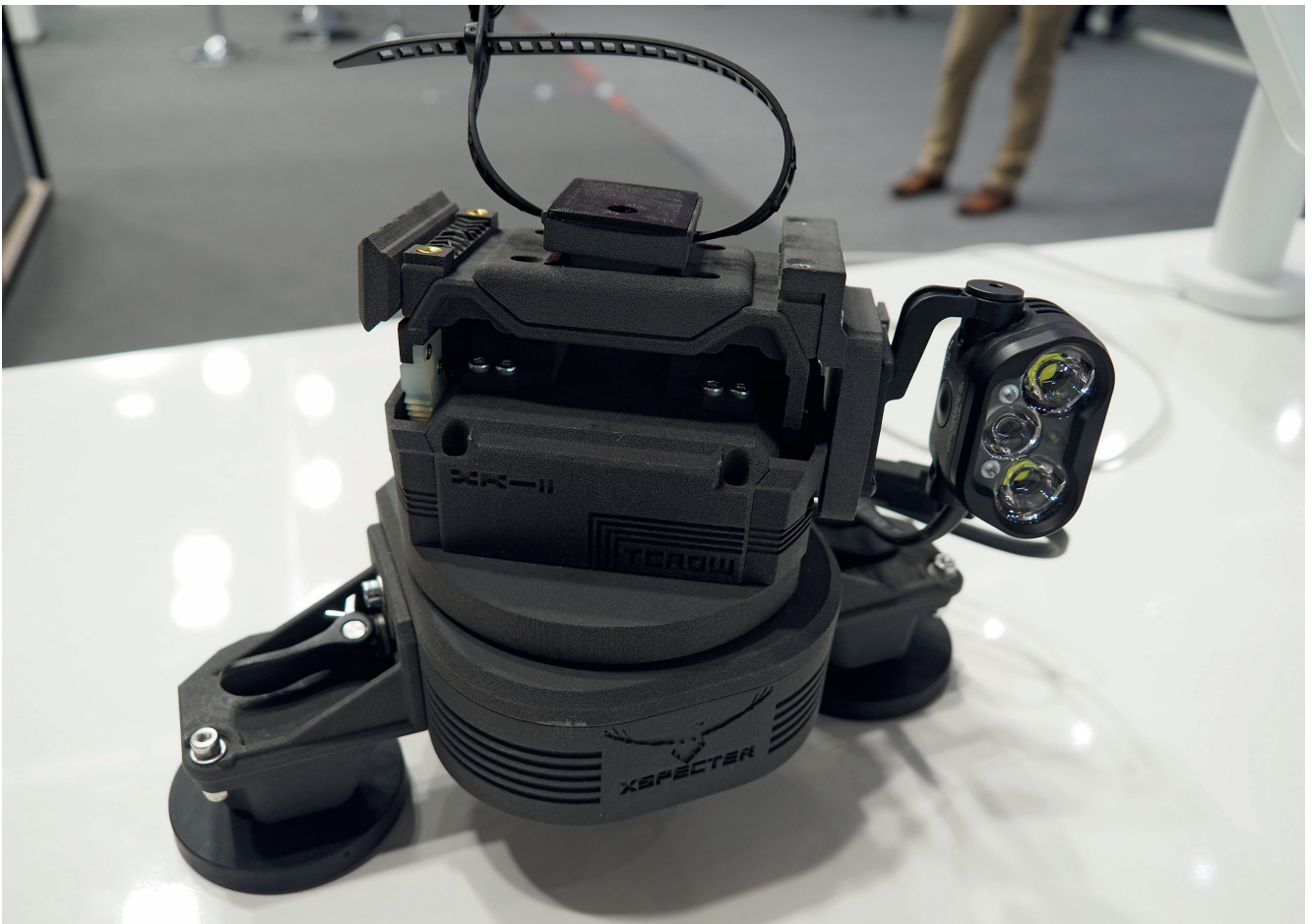
T-Crow night vision camera: except for the electronic components, the entire stand is produced additively.
